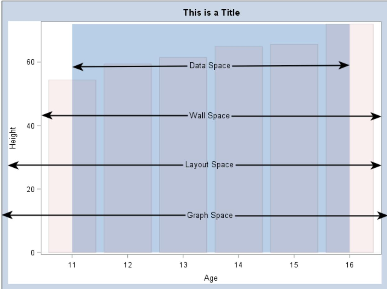
**Figure 1. Drawing Spaces for a Single-Celled Graph**
