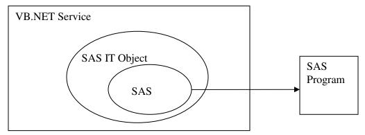
As shown above, the VB.NET service is a wrapper for the SAS object, which is a wrapper for SAS, which executes the SAS program. The entire system is loaded into the Windows Services Manager, which is part of Windows.
