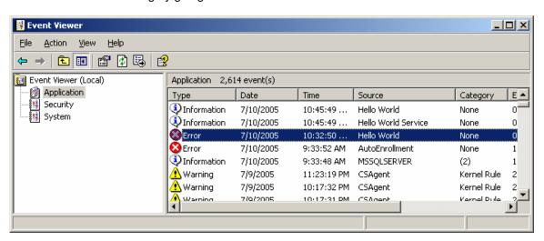
The Event Viewer displays three different logs: Application, Security, and System. The messages your service generates should all go to the Application log.
